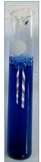
Test tubes containing: Bradford reagent with protein added. ( \lambda_{\max} ) is shifted to 595nm.
